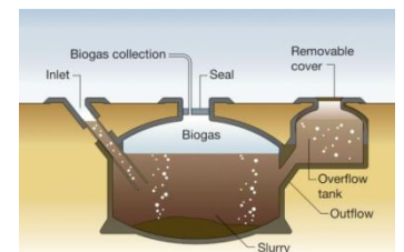
▲ Figure 1 A biogas plant
